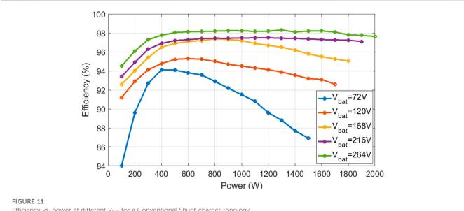
Efficiency vs. power at different V<sub>bat</sub> for a Conventional Shunt charger topology.
