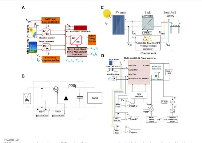
PV-Battery charge controller topology using (A) Fuzzy-based battery energy management in a hybrid solar and wind renewable system (Nagaiah and Sekhar, 2020). (B) A PWM for fast battery charging (Mehmood et al., 2016). (C) incorporates two cascaded FLC (Rkik et al., 2021). (D) A multi-port DC-DC power converter (Almutairi et al., 2021).
