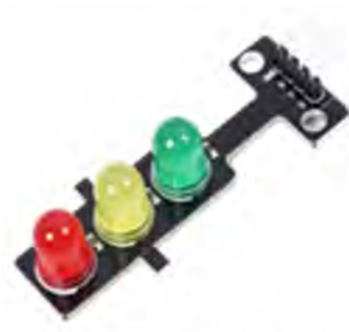
Figure 11. Traffic light module.
