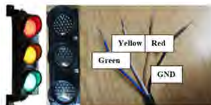
Figure 10. Traffic light and pinouts.
