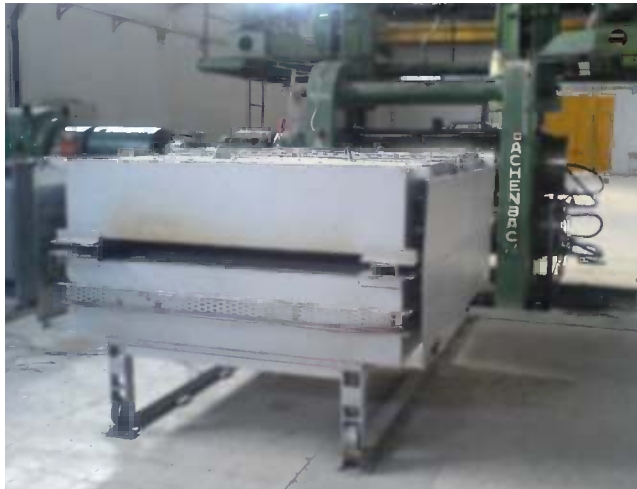
Figure 2. Photograph of industrial scale rolling mill system and furnace used for hot rolling.
