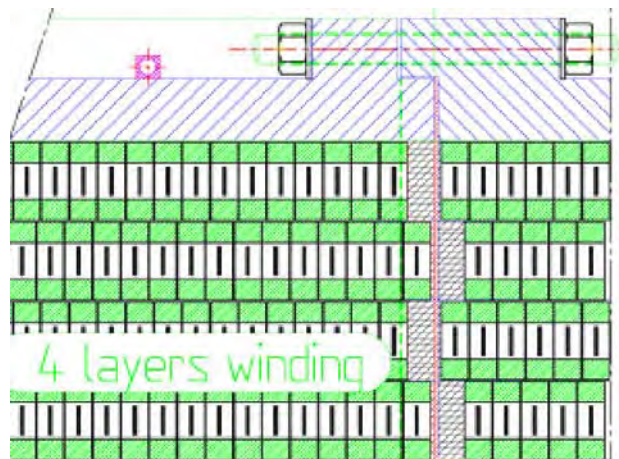
Figure 2.5: Detail of the interface region between 2 modules. In order to guarantee mechanical continuity, false turns are involved. The modules are connected through bolts and pins fixed through the outer mandrels.
