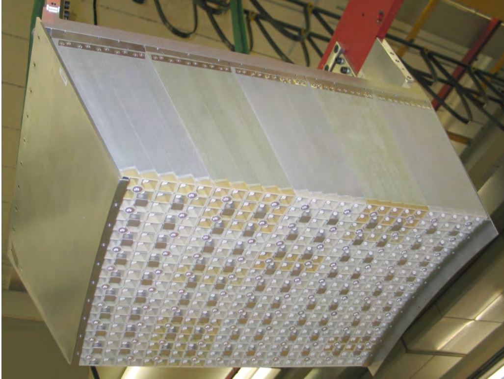
Figure 4.4: Front view of a module equipped with the crystals.
