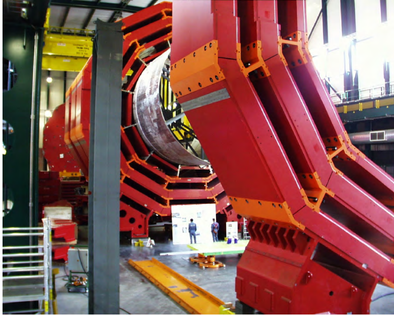
Figure 2.6: A view of the yoke at an early stage of magnet assembly at SX5. The central barrel supports the vacuum chamber of the superconducting coil. At the rear, one of the closing end cap disks is visible.
