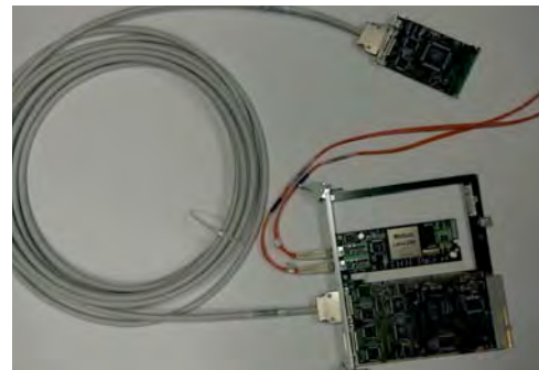
Figure 9.4: Photograph of S-link64 sender card, LVDS cable and compact-PCI FRL card with embedded LANai2XP NIC. Connected to the NIC are fibres that go to the FED Builder input switch.
