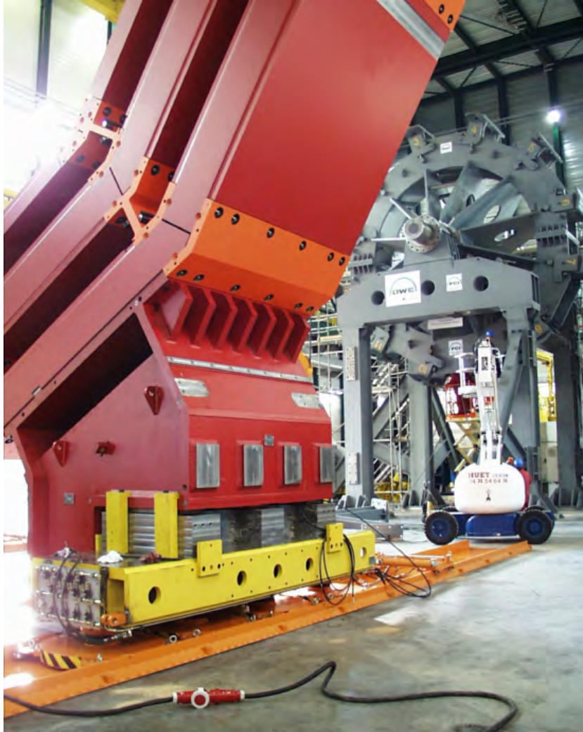
Figure 10.3: A transport beam for barrel rings with 4 air pads fixed on it.
