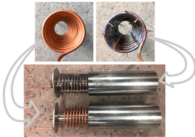
Fig. 5. Inner view of the manufactured SHCHes.
