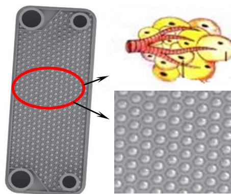
Figure 2. Design of trachea pattern compact PHE.
