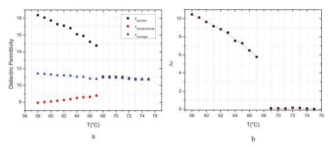
**Figure 2.** (Colour online) (a) The dielectric permittivity and (b) the dielectric of anisotropy  $\Delta \varepsilon$  of 4-propoxy-biphenyl-4-carbonitrile at 10 kHz. Solid lines are drawn as guides to the eye.
