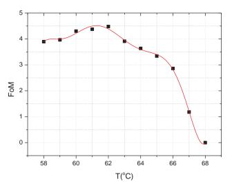
**Figure 7.** (Colour online) Temperature variation of figure of merit (FoM) at  $\lambda = 633$  nm. Solid lines are drawn as guides to the eye.
