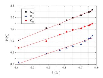
**Figure 6.** (Colour online) Variation in  $K_{ii}$  as a function of  $\Delta n$ . Solid lines are linear fit to the data points.
