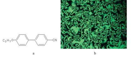
**Figure 1.** (Colour online) (a) The chemical structure of 4-propoxy-biphenyl-4-carbonitrile and (b) the photomicrograph (×100) of the schlieren texture in nematic phase at 65°C.
