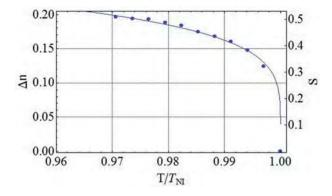
**Figure 5.** (Colour online) Optical birefringence  $(\Delta n)$  and order parameter (S) as a function of temperature. Solid lines are drawn as guides to the eye.
