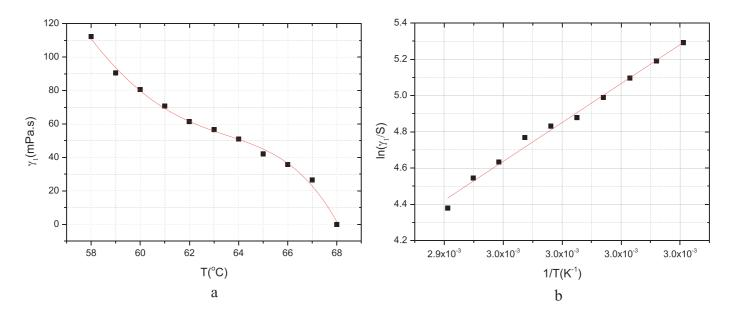
Figure 4. (Colour online) Variation of the rotational viscosity (y<sub>1</sub>) of 4-propoxy-biphenyl-4-carbonitrile as a function of temperature. Solid lines are drawn as guides to the eye.
