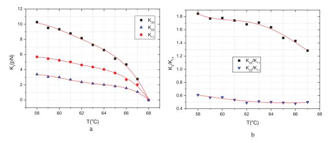
Figure 3. (Colour online) (a) Temperature dependence of elastic constants and (b) temperature variation of the elastic ratio. Solid lines are drawn as guides to the eye.
