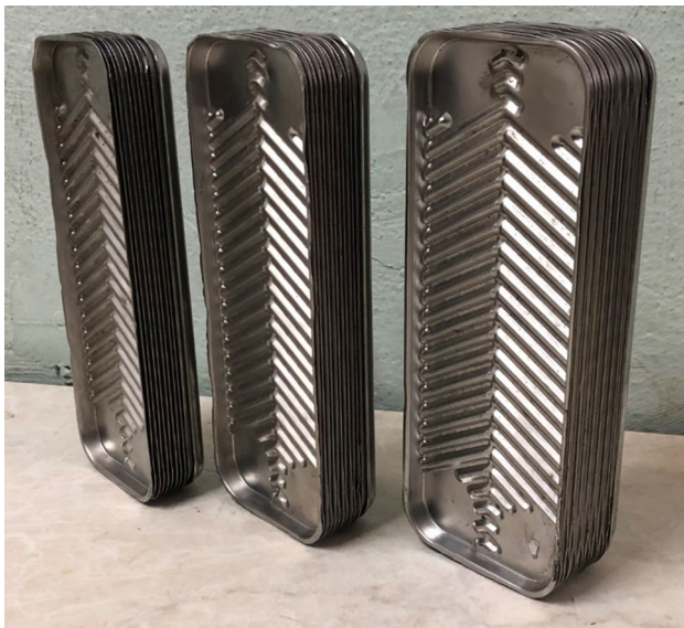
Fig. 3 A view of utilized plate-type heat exchangers
