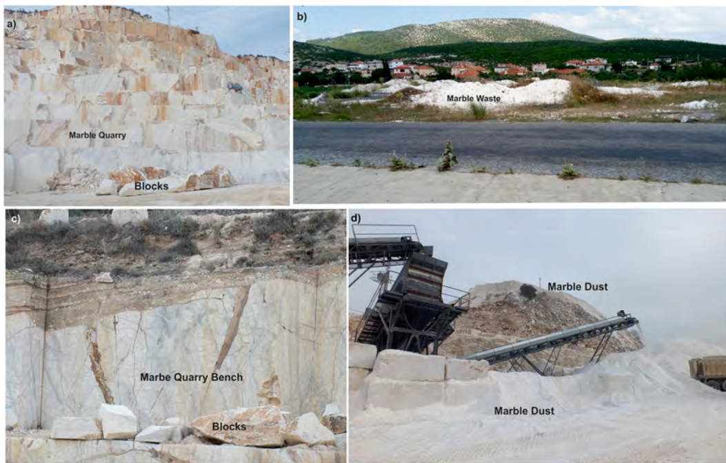
Fig. 9 (a) Field view of the marble quarry that includes 5–8-m steps. (b) Randomly dispersed marble waste including palladian, marble dust and blocks caused visual contamination. (c) Various sized residual material can be form during the mining operations;
