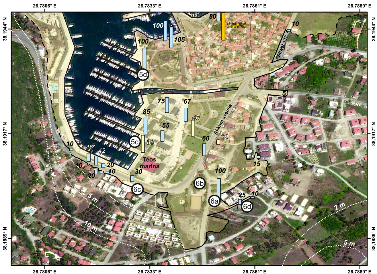
Fig. 3 The columns represent the flow depth measurements. Yellow, orange, grey and blue columns are from Yalçiner et al. (2020a, b), Doğan et al. (2020) and this study, respectively. The yellow shading corresponds to the inundated area. White circles indicate figure
