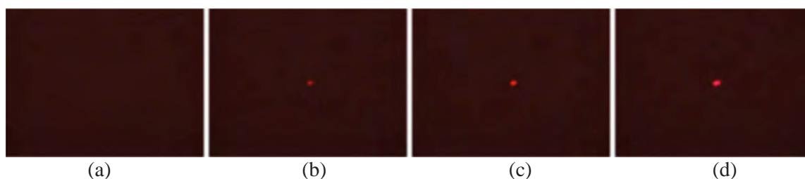
Figure 5. (Colour online) The observed laser beam images (a) without LC sample and with the sample at the applied voltage (b) 0 V_{\text{rms}} , (c) 50 V_{\text{rms}} and (d) 200 V_{\text{rms}} .
