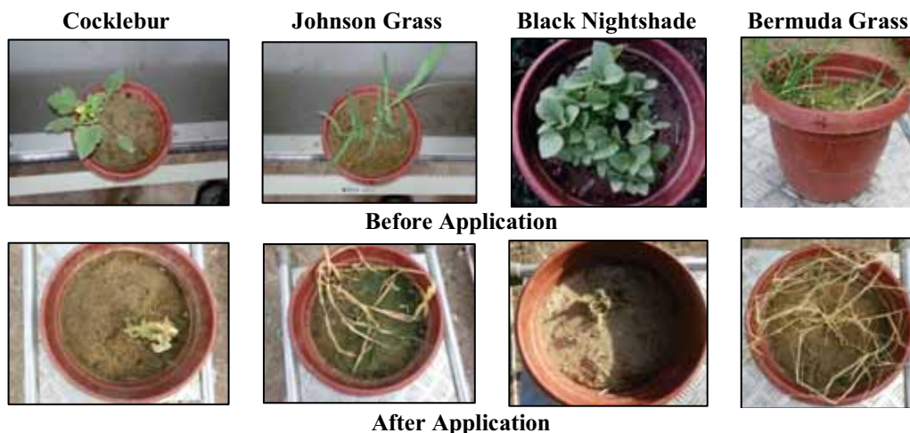
FIGURE 3 Weeds before and after the microwave application
