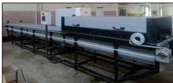
FIGURE 1 Laboratory prototype microwave oven
