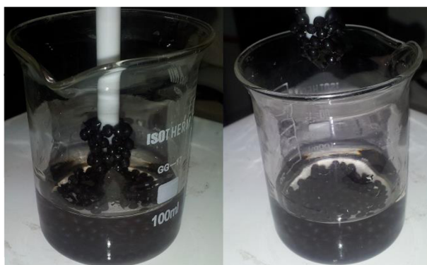
Fig. 3 The photograph of magnetic beads attracted by magnetic bar
