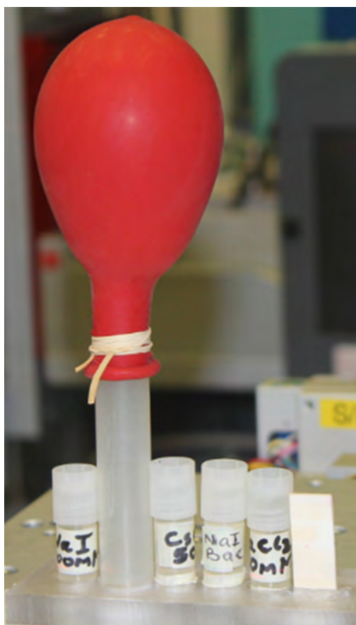
Figure 6. Subject imaged constituting of six materials: starting from left to right: NaI, Xe, CsCl, a mixture of BaCl 2 and NaI, BaCl 2 , and ‘physics bone’—simulated bone (hydroxyapatite in a plastic matrix).
